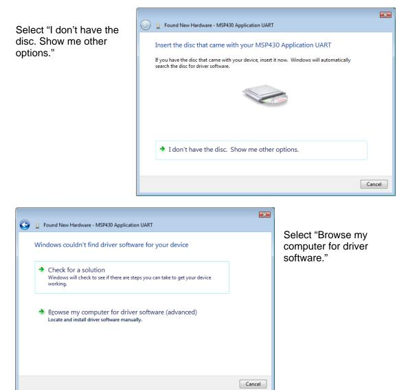
The required "inf" file will be installed together with the application. Browse to the directory of the application and select the sub directory "Drivers".
